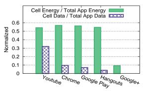
Figure 5: The fraction of data delivered by cellular versus the fraction of energy consumed by cellular for popular apps.
