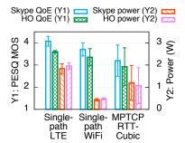
Figure 8: QoE and power consumption of VoIP under different SPTCP/MPTCP settings.
