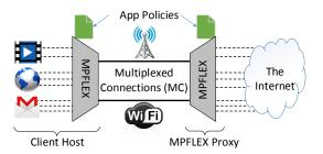
Figure 12: The MPFlex architecture.
