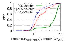
Figure 6: Throughput ratio of MPTCP (WiFi primary) to SPTCP over WiFi for 4,371 back-to-back throughput measurements for different LTE signal strength levels.
