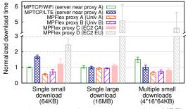
Figure 18: Case study: MPTCP applies multipath to all traffic, while MPFlex does that selectively based on user policy.
