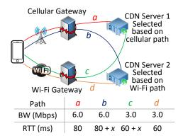
Figure 9: Example: CDN sever selection over multipath.
