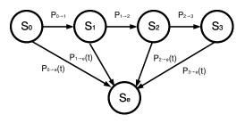
Figure 18: The time-inhomogeneous Markov process (TIMP) that models the Data\_Stall recovery process in Android, where the transition probabilities among the five states are also impacted by the elapsed time (*t*).
