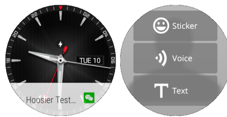
Figure 9: Left : a WeChat card showing at the bottom of the screen. Right : reply to a message using the WeChat app on watch.
