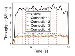
Fig. 3. Uplink test logic of SpeedTest.
