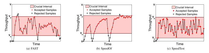
Fig. 5. Undesirable scenarios where the accepted samples within the crucial interval do not manifest sufficient concentration.
