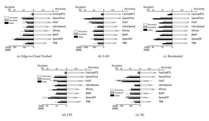
Fig. 8. Test duration, data usage, and test accuracy of FastUpBTS, compared with seven representative BTSes under diverse networks. Note that the error bars indicate the standard deviations rather than min-max deviations.
