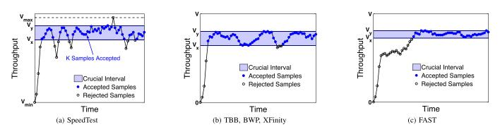
Fig. 4. Common scenarios where the true samples fall in a crucial interval during an uplink bandwidth test.
